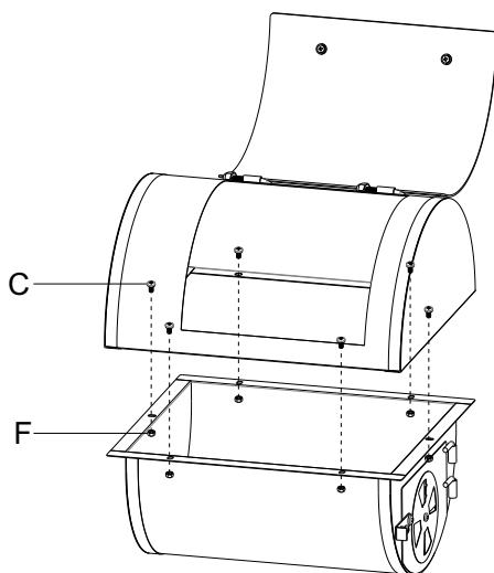
Please install and fix the ONE SIDE (Front) two holes to match the lid and fire bowl ,
