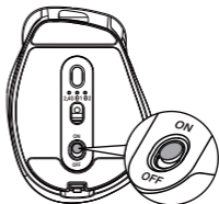
Open Power Switch
